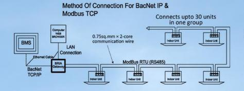
Connects upto 4 groups of 30 units with one **BRIA Gateway** and further connect to your BMS system or connects to your computer and monitor using web browser **BRIA Gateway** can also be used for Modbus RTU connection for upto 3 groups of 30 units with one Gateway. (one network adaptor is required for each unit to make it compatible for above network structure)
