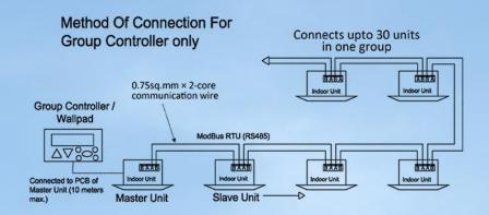
Connects upto 30 units with one **Group Controller / Wallpad**, able to set parameters of individual units in one group Set temperature locking function with **Wallpad** (standard 27degC; can be changed as per requirement)
