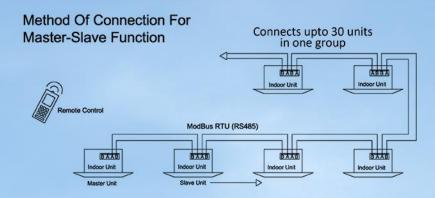
Connect upto 30 units in one group, making one unit as **Master unit** and other units as **Slave unit**. All Slave units will follow master unit if any changes of parameter is made in master unit (one network adaptor is required for each unit to make it compatible for above network structure)
