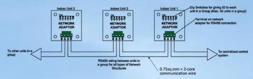
Above connection would be same in a group for every network structures Connects upto to 30 units in group Set each units in a group with different ID using "Dip Switches" (one network adaptor is required for each unit in all of above network structures)
