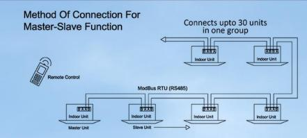
Connect upto 30 units in one group, making one unit as **Master unit** and other units as **Slave unit**.
