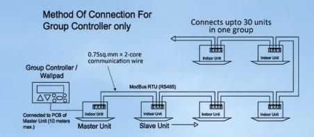
Connects upto 30 units with one **Group Controller / Wallpad**, able to set parameters of individual units in one group Set temperature locking function with **Wallpad** (standard 27degC; can be changed as per requirement)
