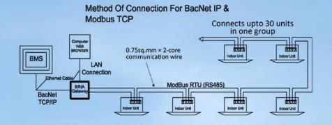
Connects upto 4 groups of 30 units with one **BRIA Gateway** and further connect to your BMS system or connects to your computer and monitor using web browser **BRIA Gateway** can also be used for Modbus RTU connection for upto 3 groups of 30 units with one Gateway. (one network adaptor is required for each unit to make it compatible for above network structure)
